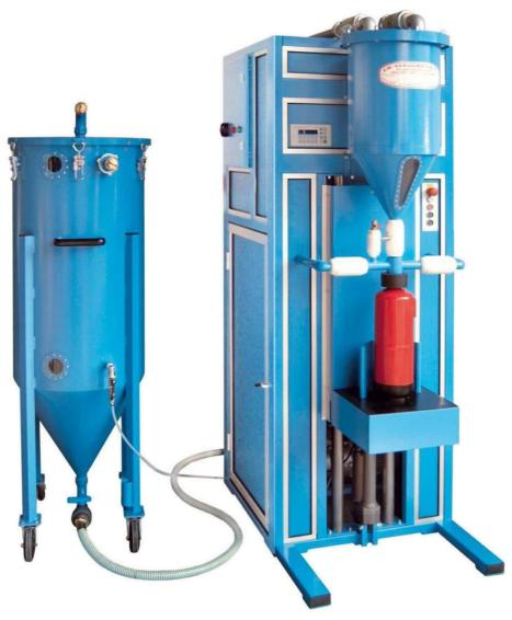
The unit operates within the filling tolerance indicated in the EN3 standards. Adjustment of the value of the filling weight has to be effected at the scale display; adjustment of the filling parameters depending on extinguisher type are effected by the text display. Height adjustment of the weighing platform takes place by screw-drive.
