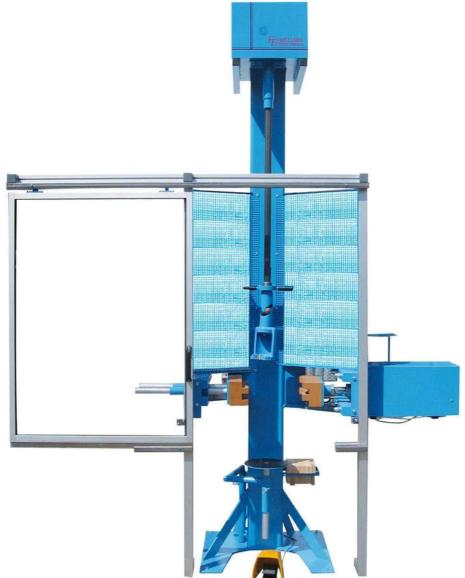
The unit has torque adjustment (0-925 Nm) and torque speed regulation (0-30 rpm). The automatic cut-off mechanism is implemented using torque control. The unit is equipped with a sliding guard door and a perforated grid protective wall at the rear.
