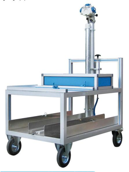
The trolley is fitted with two steering/ braking wheels and two fixed wheels. The wheels have Aluminium rims and solid rubber tyres to ensure the trolley has minimal rolling resistance and is easy to manoeuvre despite its weight even on rough ground. The single wheel load is 400 kg.
