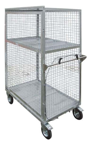
The trolley is fitted with 2 steering/braking wheels and two fixed wheels. The wheels have Aluminium rims and solid rubber tyres to ensure the trolley has minimal rolling resistance and is easy to manoeuvre despite its weight even on rough ground. The single wheel load is 400 kg.
