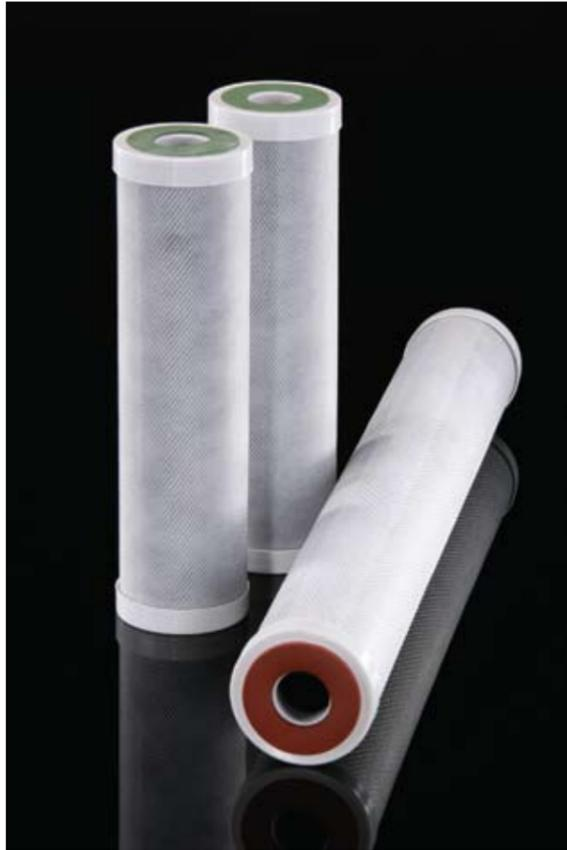
CARBOFLOW MX cartridges are offered in both high efficiency and general grades. They consist of bituminous coal sourced carbon, extruded together with an FDA listed thermoplastic binder, to produce an extremely porous yet rigid structure.
